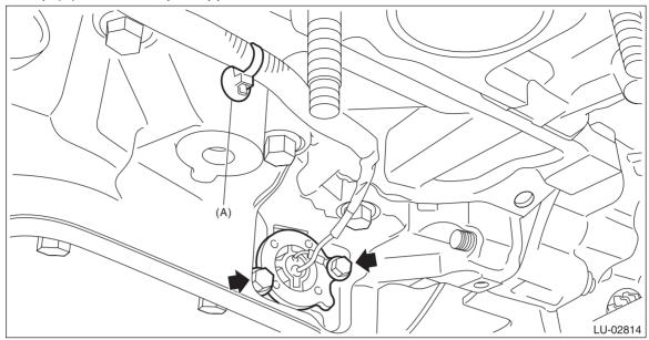
8) Remove the bolts which secure oil pan upper to cylinder block, and remove the oil pan upper.
