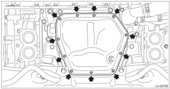
7) Insert an oil pan cutter blade into the gap between oil pan upper and oil pan, and remove the oil pan.
